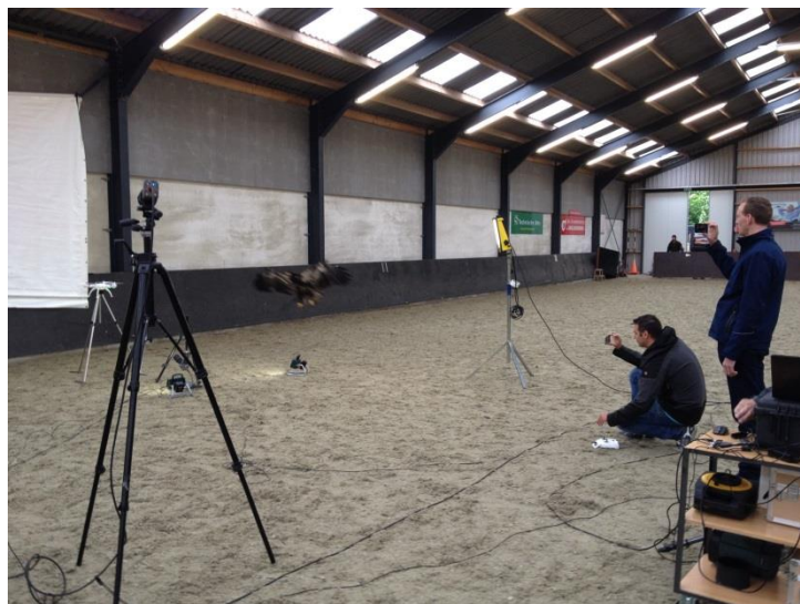
Figure 17: Test set-up and approaching bird during indoor drone intercepts.
