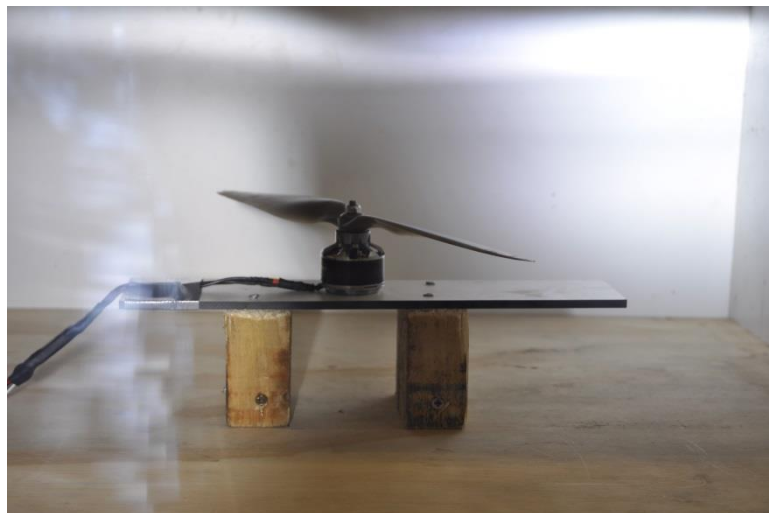
Figure 8: APC nylon propeller driven by a brushless DC-motor, shown in safety box.
