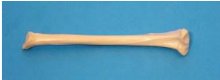
Figure 4: Feline tibia surrogate made from a solid foam [Synbone, 2016].
