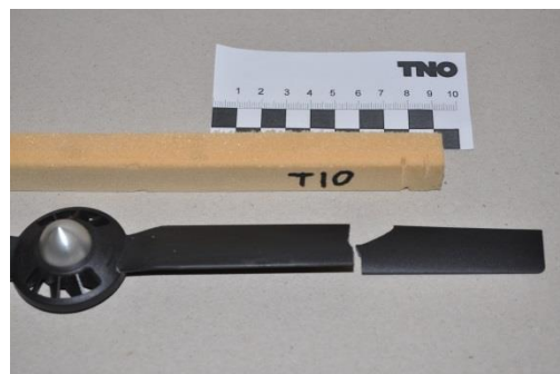
Figure 10: High density PVC foam: results for test number #10
