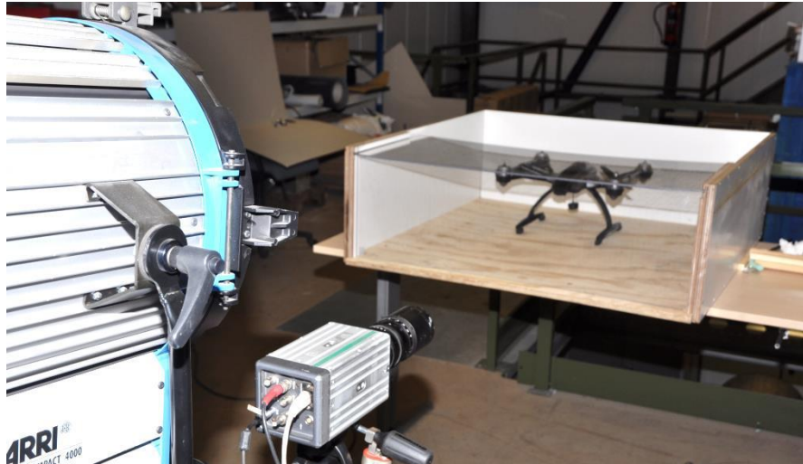
Figure 7: Test set-up with light source, high-speed camera and safety box around the YUNEEC Q500G Typhoon Quadcopter.
