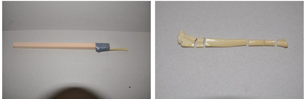
Figure 11: Feline tibia surrogate before and after test #13.
